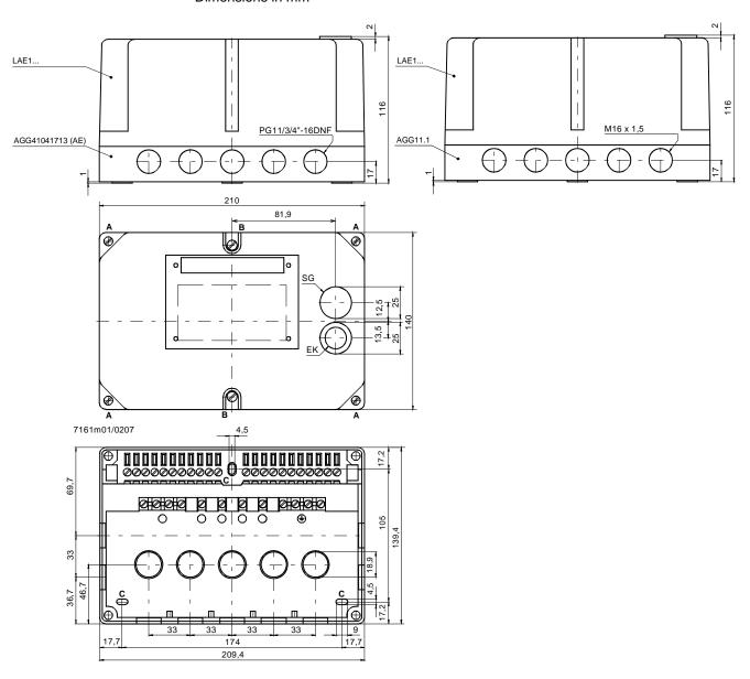
To remove the LAE1... from its plug-in base, it is **merely** necessary to loosen the 4 screws  $^{\diamond}$ A».
